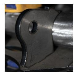
5. Tack weld all components to the frame in multiple places. Remove clamps.
