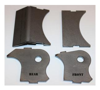
4. Install the tabs into the keyways on the diff plate.
